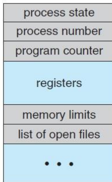
Figure 3-2 Process control block (PCB)
