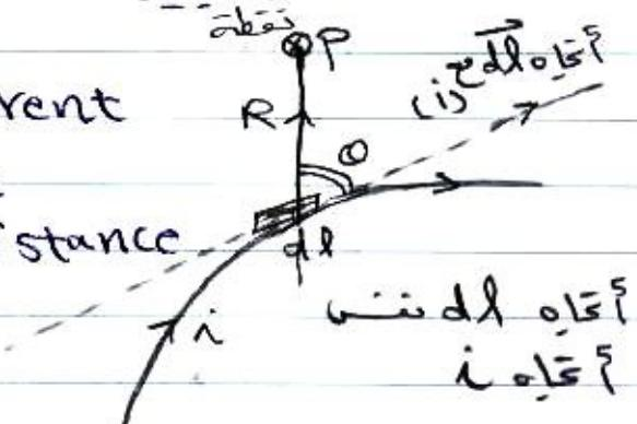
The wire is to be divided into short elements of ( $dl$ ) each element setup a field ( $dB$ ) of all point of space and the field of the entire circuit at any point is the resultant of the fields of all the elements of the circuit.
