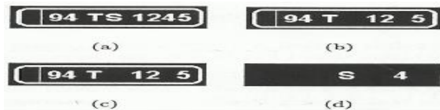
Figure 2.10: a) input image1 a(x,y) b) input image2 b(x,y) c) a(x,y) \oplus b(x,y) d) a(x,y) \otimes b(x,y)
