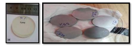
Figure 4: Photograph of Thermal conductivity Test Specimens for Epoxy and Epoxy/ Aluminum composites.
