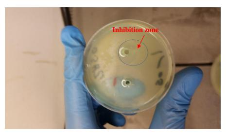
Figure 9. Inhibition zone of 25×15 mm using built-in Nickel electrodes at 0.5 Hz for 30 minutes.
