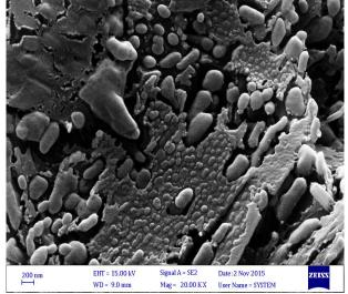
Figure (10). SEM pictures of polymeric mixture G nanocomposite.
