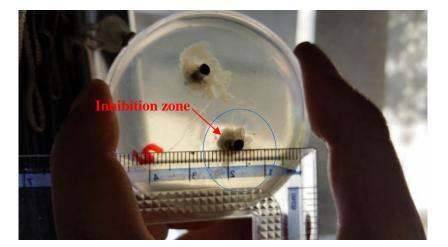
Figure 12. Inhibition zone of 33×24 mm using built-in Nickel electrodes at 100 KHz for 30 minutes.
