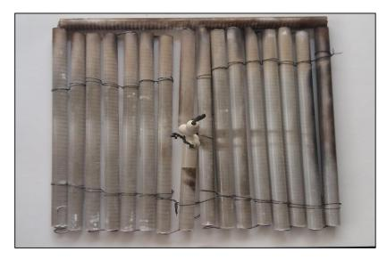
Figure 1. Home-made electrical heater using tungsten wire and quartz tube.
