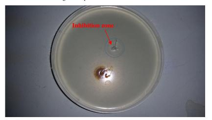
Figure 8. Inhibition zone of 5 mm burning trace at anode side using movable Nichrome electrodes at 3 KHz for 10 minutes.
