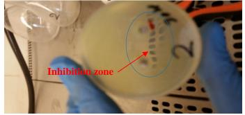
Figure 10. Inhibition zone of 20×15 mm, using built-in Nickel electrodes at 30 Hz for 30 minutes.
