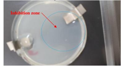
Figure 13. Inhibition zone of 35×30 mm, closely total bactericidal effect using built-in Titanium electrodes at 120 KHz for 30 minutes.
