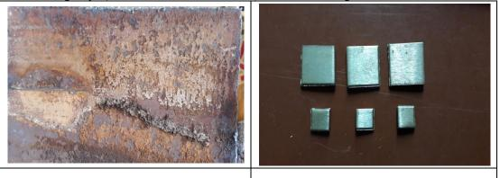
Figure 1. St-37 alloy exposed to corrosion
