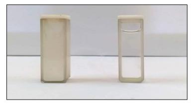
Figure 3. Methanol and Colloidal suspensions of TiO<sub>2</sub> at 1.32 J/cm<sup>2</sup> pulse laser fluence from left to right.
