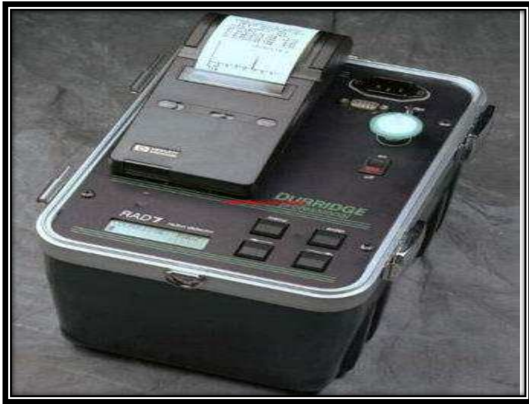
Fig (2 - 3) : The RAD-7™ electronic continuous monitor of radon with a HP printer mounted for immediate printing of results [80].
