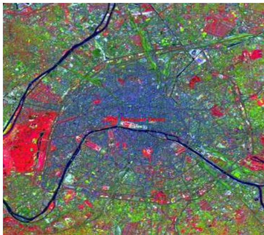
Figure (2-10) Finding Vegetation in a Multispectral image [82].
