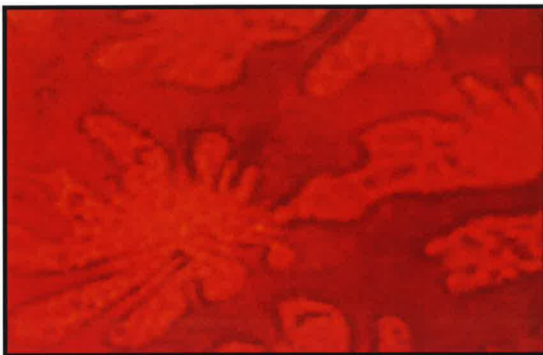
Figure (3-48): Cross polarizing optical textures of smectic B phase for compound [XIV] b at 80 °C
