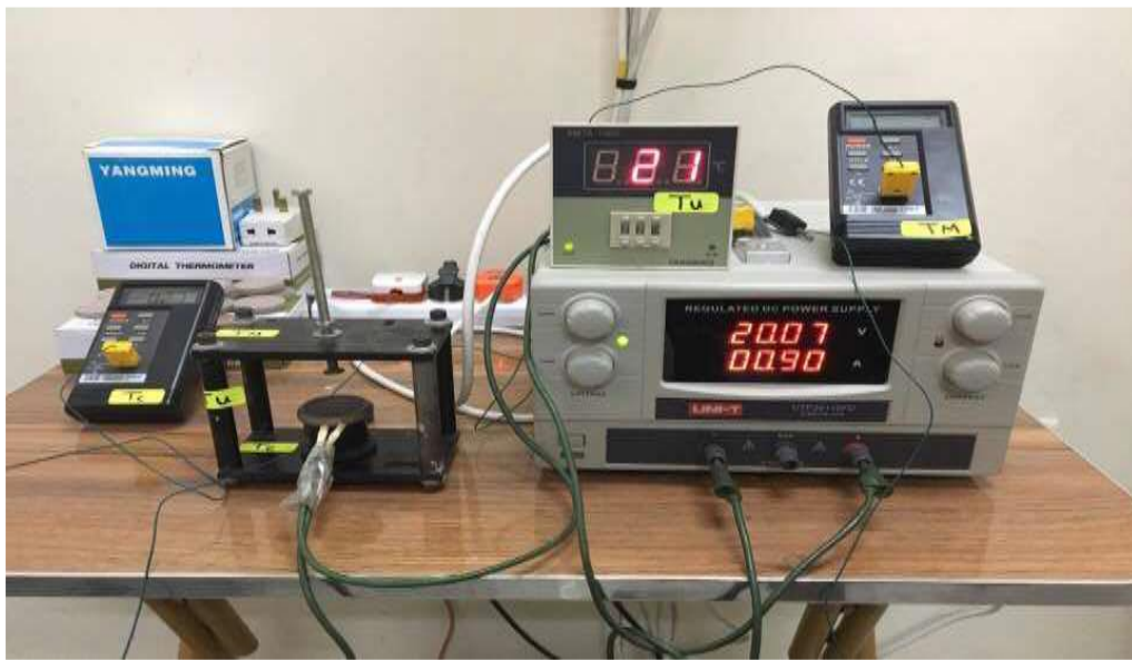
Figure (3-8) shows thermal conductivity test device.
