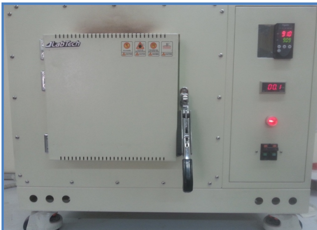
Figure (3-4) image of the furnace sintering
