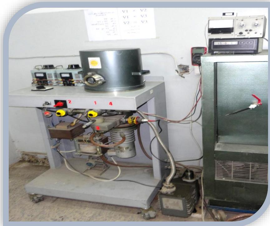
***Figure (3-2) vacuum evaporation system***
