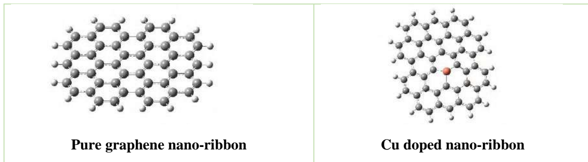
Fig.1. Geometrical structural for pure and doped nano-ribbon.
