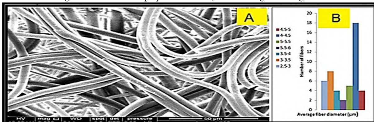
Figure 5. 30 wt.% EPS prepared at 18KV , A:SEM image B:Histogram.
