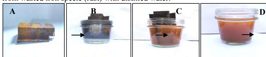
Figure 2. shows the steps for preparation a spent iron extract, A) iron specie, B) iron specie with distilled water before exposes for sunlight, C) spent iron extract after exposes for sunlight, and D) spent iron extract.
