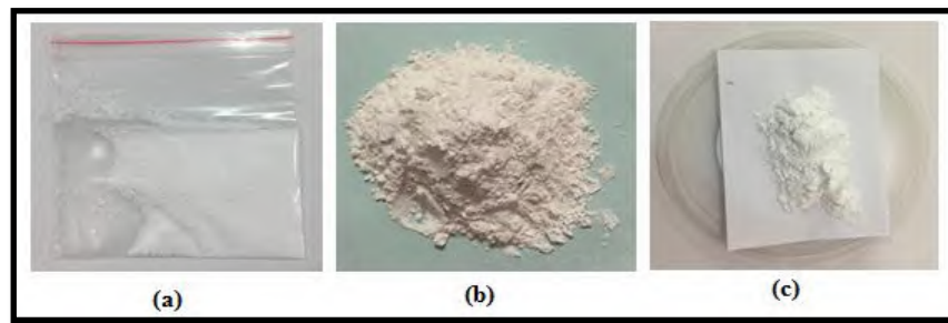
Figure 1. The materials used as reinforcement in biocomposite materials: (a) Nanohydroxyapatite; (b) Hydroxyapatite prepared from fish bones; (c) Hydroxyapatite prepared from natural egg shells.
