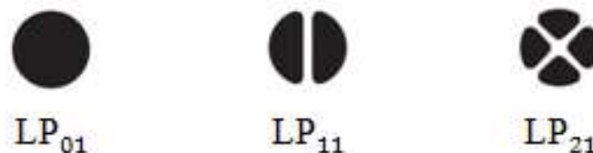
Figure 1. Intensity profiles for the three lowest linearly polarized (LP) modes [6].
