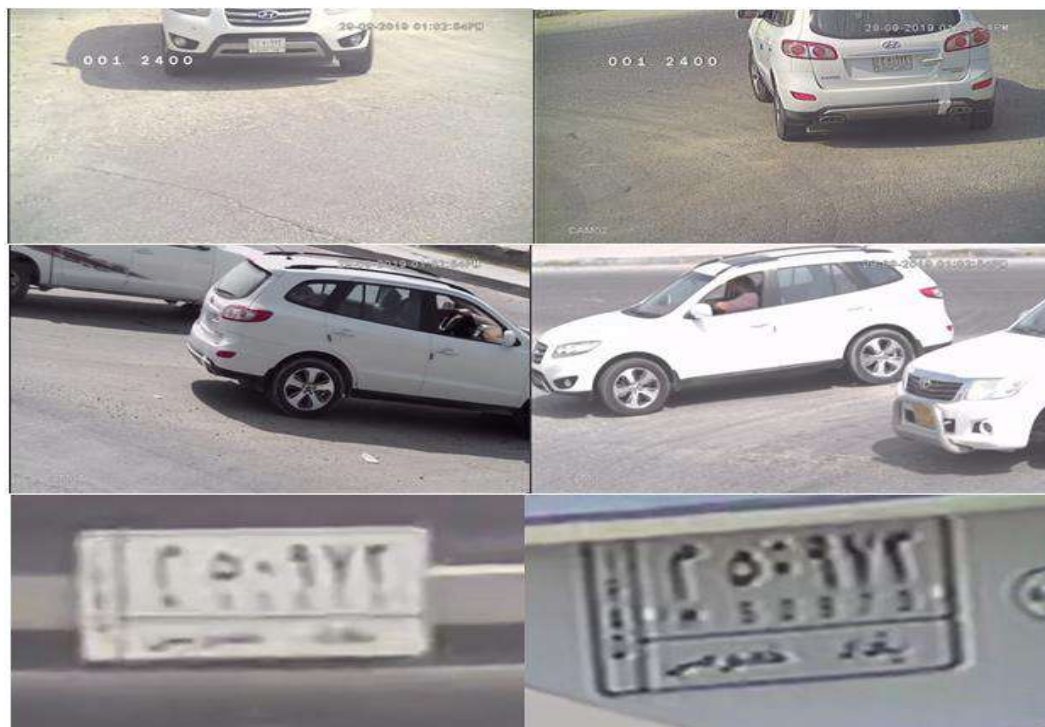
Figure 8. Capturing platelets of violated vehicle (2276.jpg) that detected by R1. First row: two frames of PTZ cameras on optical motorized zone. Second row: two frames of motorised cameras on optical motorized zone. Third row: zoomed PTZ frames of first row. Note that platelets license form in Arabic language and numbers (50972 M / Baghdad, Iraq).
