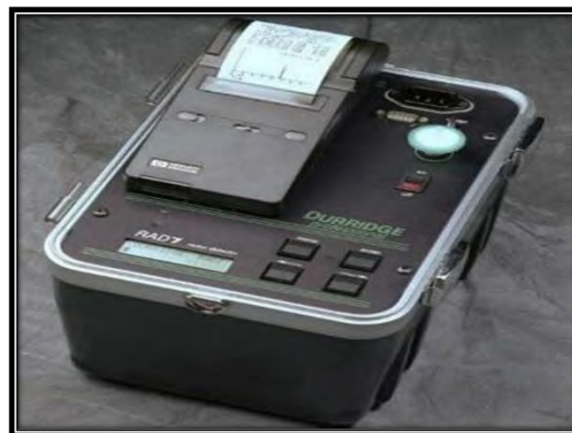
Figure 2. The durrIDGE RAD-7 electronic continuous radon monitor with an HP printer mounted for immediate printing of results.
