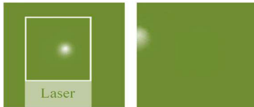
Fig. 3. An illustration of the regional center image and the incomplete laser spot image.
