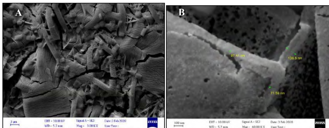
Figure 5. A-B FE-SEM images shows the results of iron oxide NPs prepared from rust iron extract with rose plant extract, at 300 °C.
