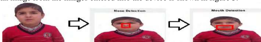
Figure 2. Defining the mouth area by shifting and enlarging the square that determines the nose
