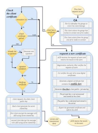
Figure 1 .The Block Diagram of the Proposed Model
